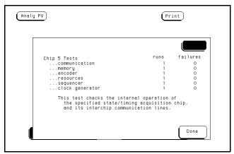
7 Select Board Tests, then select Run. When the Board Tests are finished, select Done.
